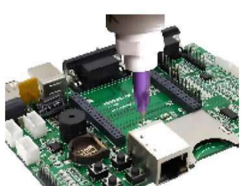
Chip corner reinforcement (non-thermally cured)
